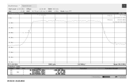
Emission Occupied Bandwidth 802.11ac 5260MHz
