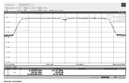
Emission Occupied Bandwidth 802.11n 40MHz 5230MHz
