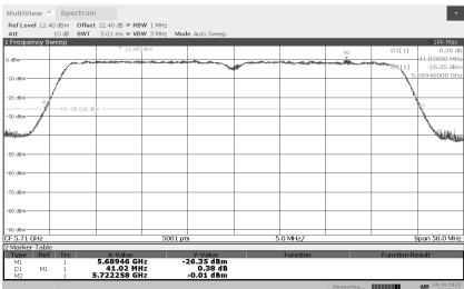
Emission Occupied Bandwidth 802.11n 40MHz 5755MHz
