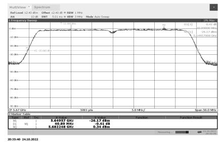
Emission Occupied Bandwidth 802.11n 40MHz 5710MHz
