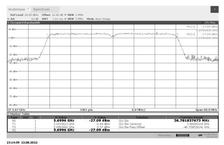
99% Occupied Bandwidth 802.11n 40MHz 5710MHz
