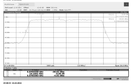
Emission Occupied Bandwidth 802.11ac 5580MHz
