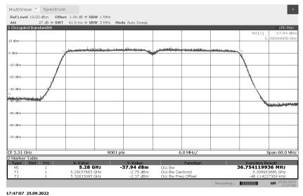
99% Occupied Bandwidth 802.11ac 40MHz 5510MHz
