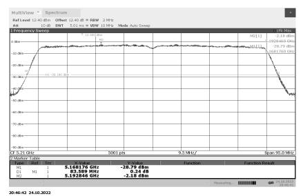
Emission Occupied Bandwidth 802.11ac 80MHz 5290MHz
