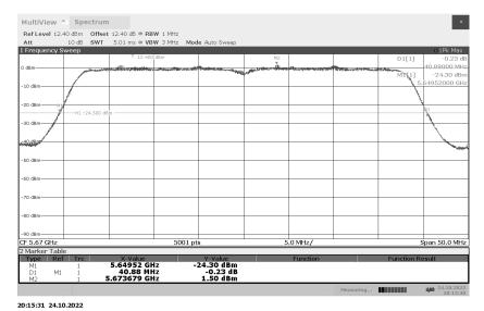
Emission Occupied Bandwidth 802.11ac 40MHz 5710MHz
