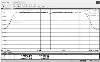
Emission Occupied Bandwidth 802.11ac 40MHz 5755MHz
