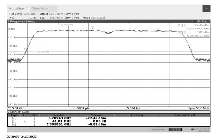
Emission Occupied Bandwidth 802.11n 40MHz 5510MHz
