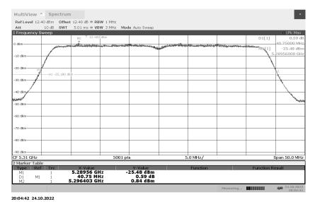
Emission Occupied Bandwidth 802.11ac 40MHz 5510MHz
