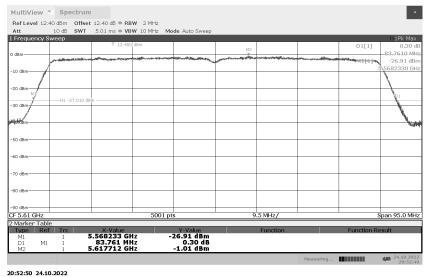
Emission Occupied Bandwidth 802.11ac 80MHz 5690MHz
