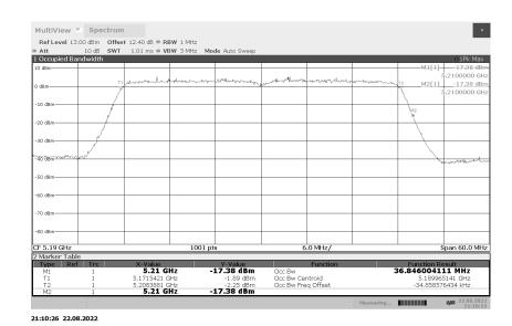
99% Occupied Bandwidth 802.11ac 40MHz 5230MHz
