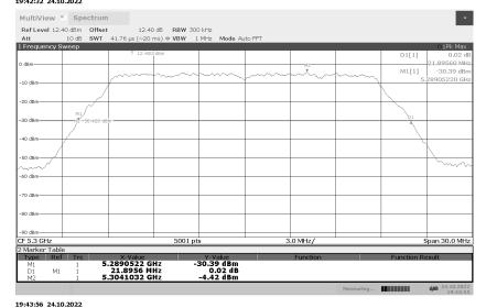
Emission Occupied Bandwidth 802.11ac 5300MHz
