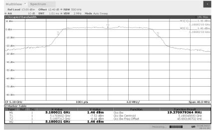
Emission Occupied Bandwidth 802.11ac 5180MHz
