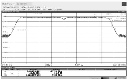
Emission Occupied Bandwidth 802.11n 40MHz 5550MHz
