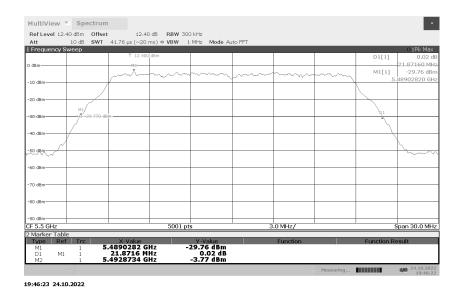
Emission Occupied Bandwidth 802.11ac 5500MHz
