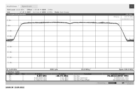
99% Occupied Bandwidth 802.11ac 80MHz 5775MHz
