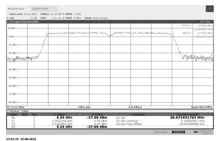
99% Occupied Bandwidth 802.11n 40MHz 5510MHz
