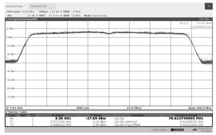
99% Occupied Bandwidth 802.11ac 80MHz 5610MHz
