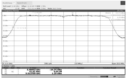
Emission Occupied Bandwidth 802.11ac 40MHz 5550MHz
