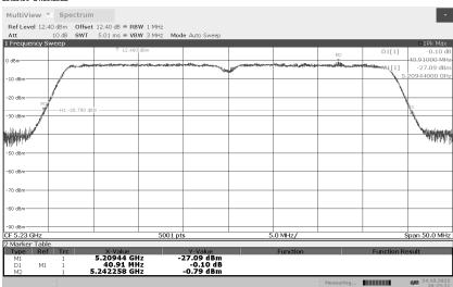
Emission Occupied Bandwidth 802.11n 40MHz 5270MHz
