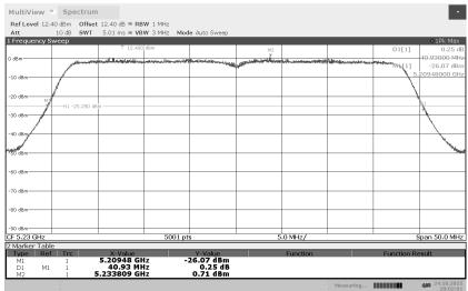
Emission Occupied Bandwidth 802.11ac 40MHz 5270MHz
