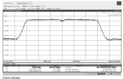
99% Occupied Bandwidth 802.11ac 40MHz 5710MHz
