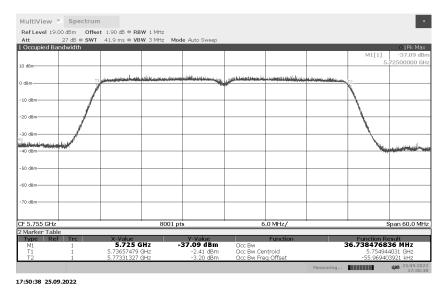
99% Occupied Bandwidth 802.11ac 40MHz 5795MHz
