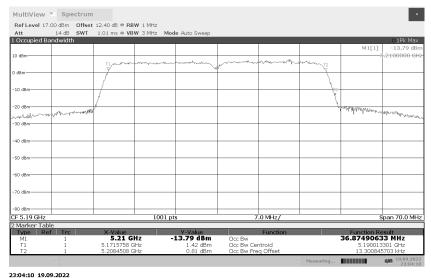
99% Occupied Bandwidth 802.11n 40MHz 5230MHz
