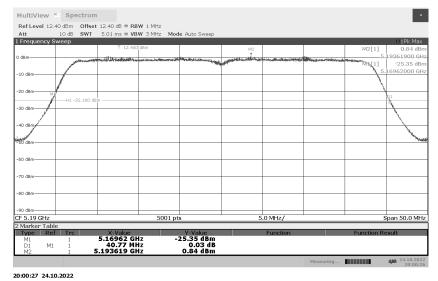
Emission Occupied Bandwidth 802.11ac 40MHz 5230MHz
