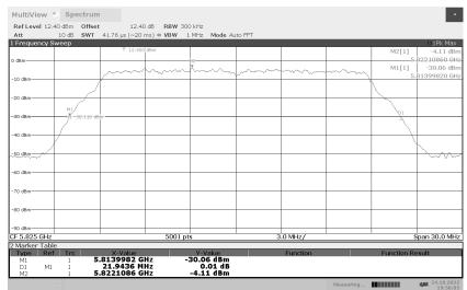
Emission Occupied Bandwidth 802.11ac 5825MHz
