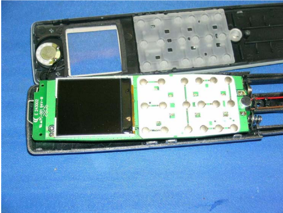
Handset Main PCB display side
