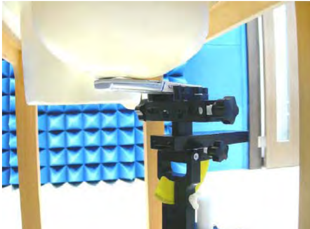
Figure 14. Right Head SAR Test Setup (Cheek)
