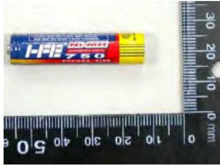
Figure 2. Battery(Ni-MH 1.2V 700mAh )
