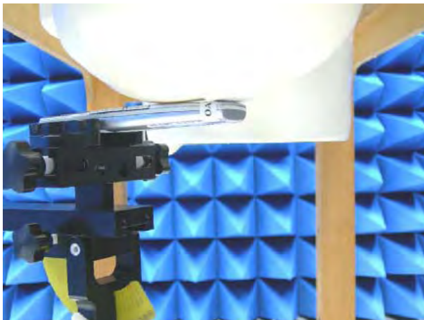
Figure 16. Left Head SAR Test Setup (Cheek)
