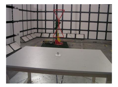
Radiated Emission - Rear View (30-1000MHz)
