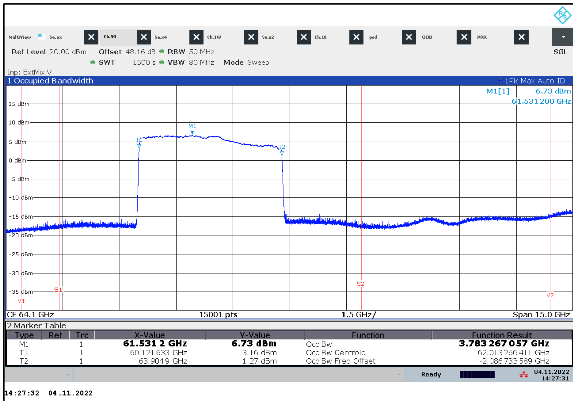
Plot 65: Occupied bandwidth, +20 °C / V nom
