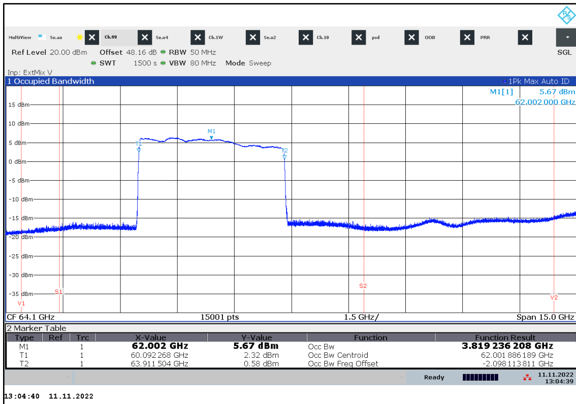
Plot 71: Occupied bandwidth, +85 °C / V nom
