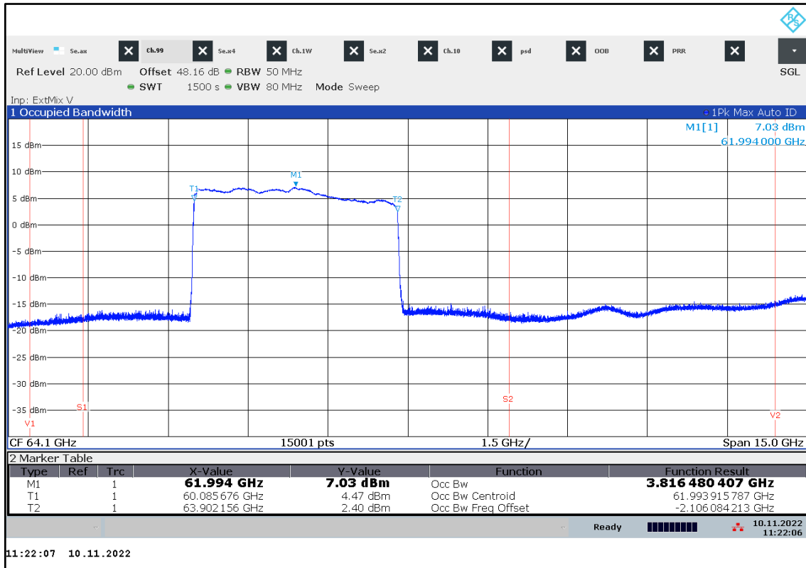
Plot 69: Occupied bandwidth, +40 °C / V nom
