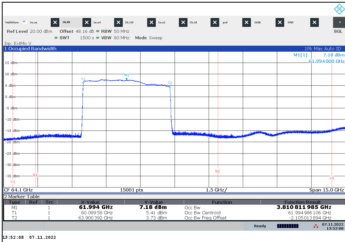
Plot 63: Occupied bandwidth, 0 °C / V nom
