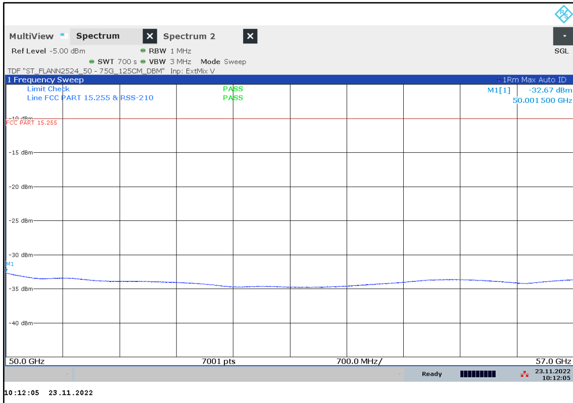
Plot 39: 50 GHz – 57 GHz, CW F mid
