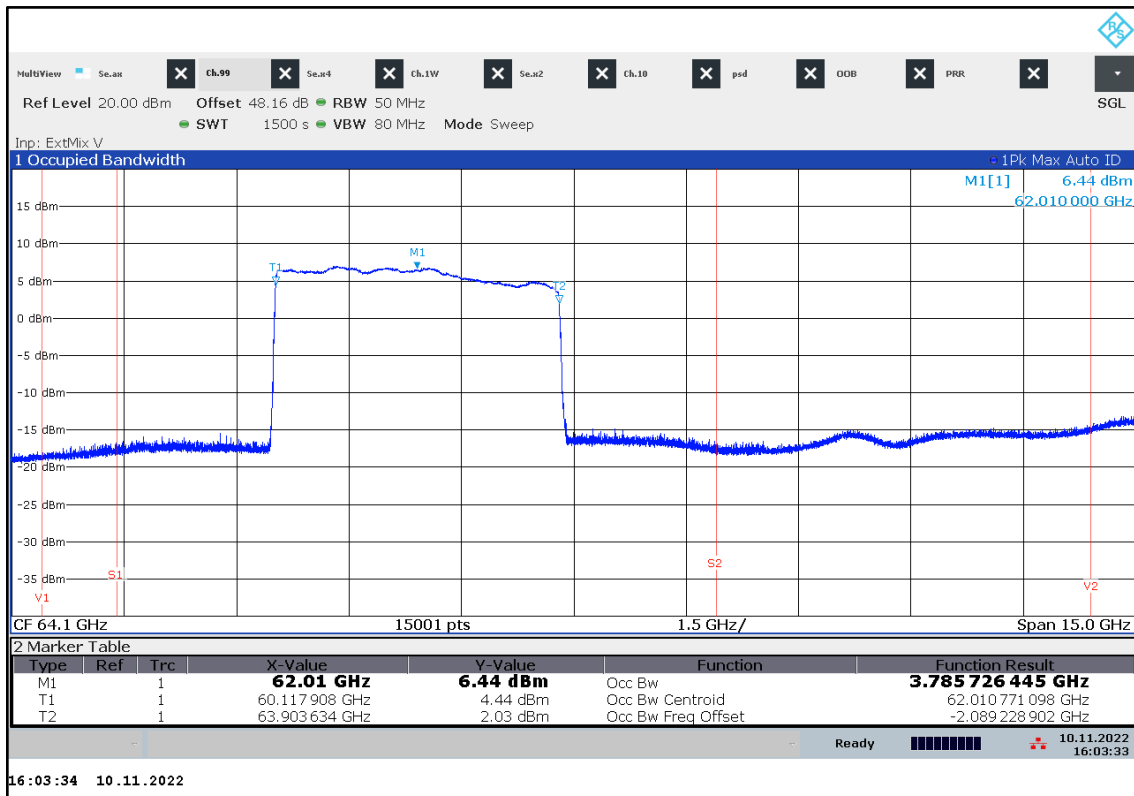
Plot 69: Occupied bandwidth, +40 °C / V nom
