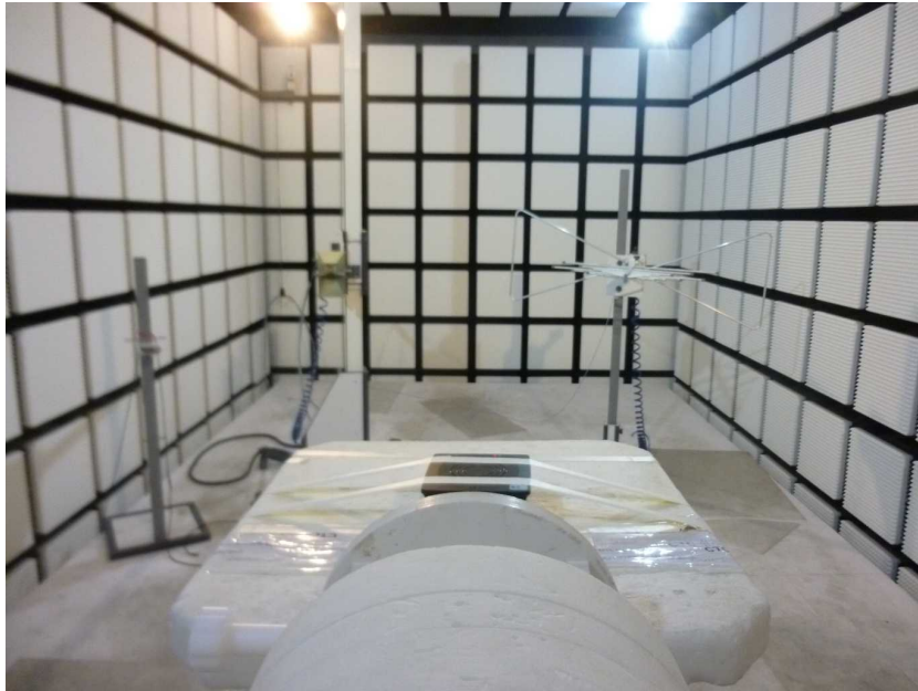
Photo 5: EUT at the anechoic chamber, test setup without tag
