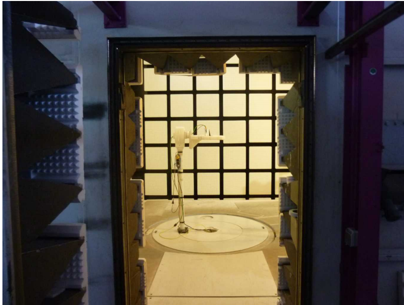
Photo 7: EUT at the anechoic chamber, test setup with tag in 20 cm distance
