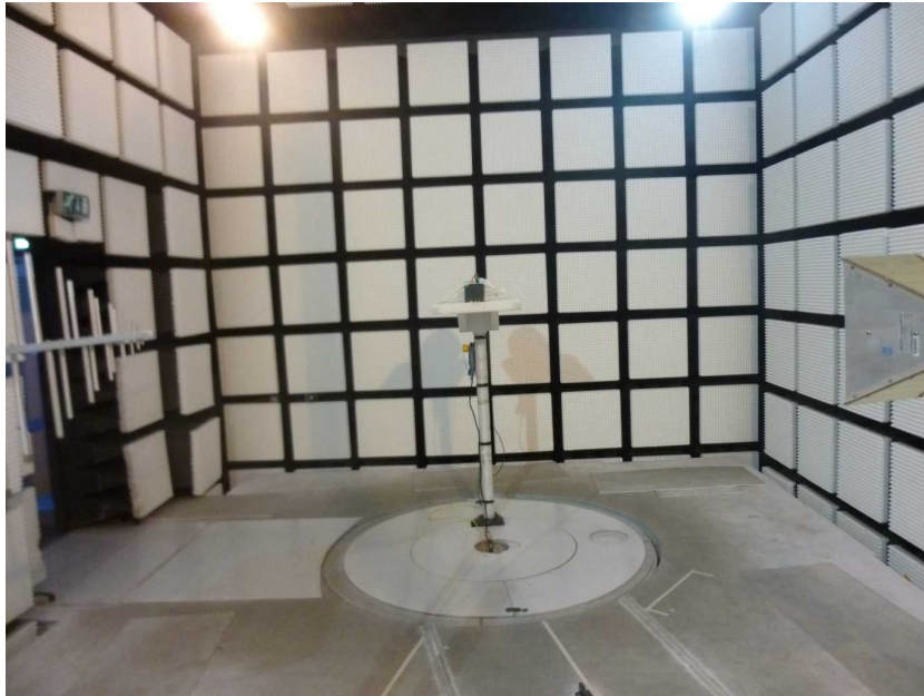
Photo 13: EUT at the anechoic chamber, test setup with tag in 20 cm distance
