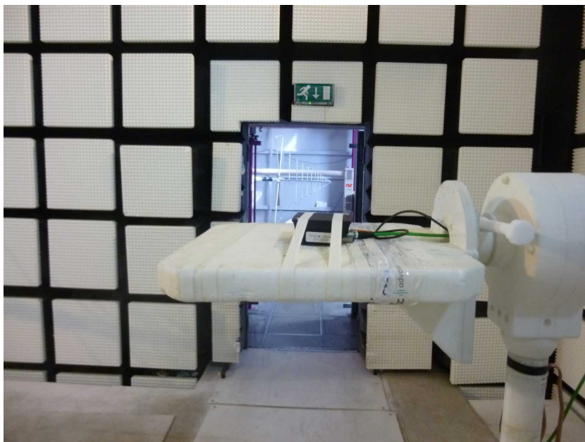
Photo 4: EUT at the anechoic chamber, test setup without tag
