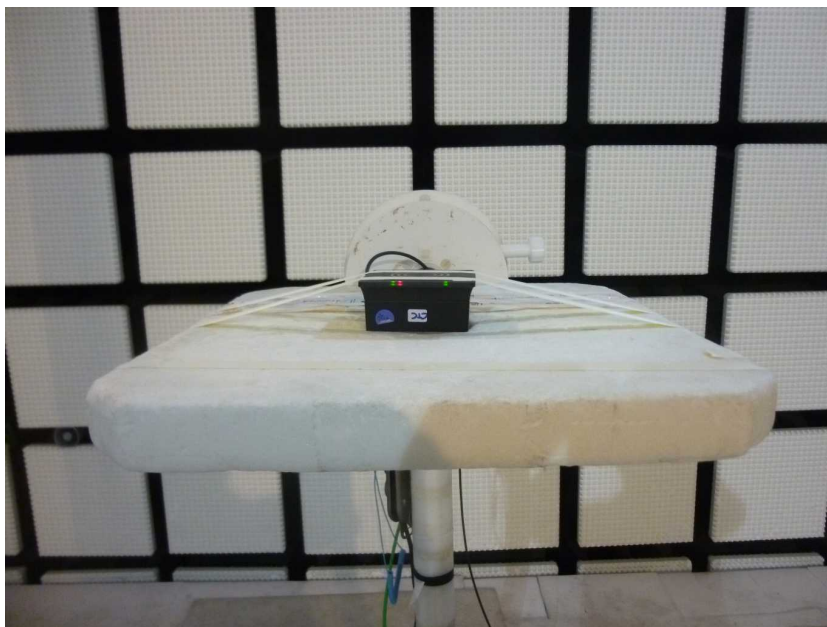
Photo 2: EUT at the anechoic chamber, test setup without tag
