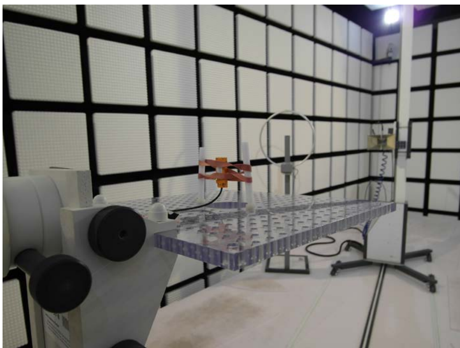
Photo 2: Test setup for radiated measurement from 9kHz to 30MHz
