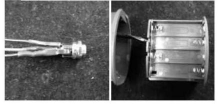
2) PLACE A 12V BATTERY INTO TRANSMITTER.
