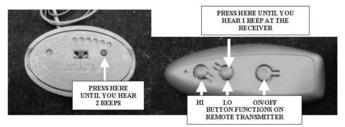
5) TO OPERATE THE SYSTEM WITHOUT REMOTE TRANSMITTER PUT RECEIVER SWITCH TO THE FAR RIGHT (ON) POSITION. THIS WILL TURN THE SYSTEM ON. YOU WILL NOT HAVE THE HI/LO FUNCTION ON THE GAS VALVE WITH
