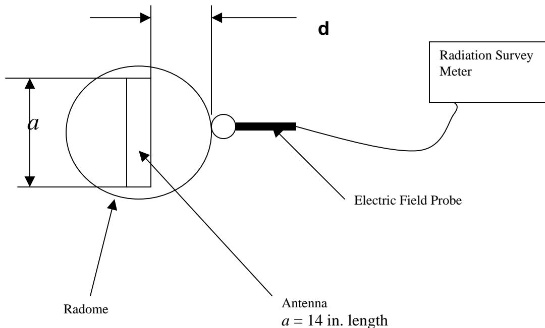
The equipment under test is perimeter surveillance radar that rotates continuously for 360 degrees in one direction at the rate of 1.08 seconds per turn.
