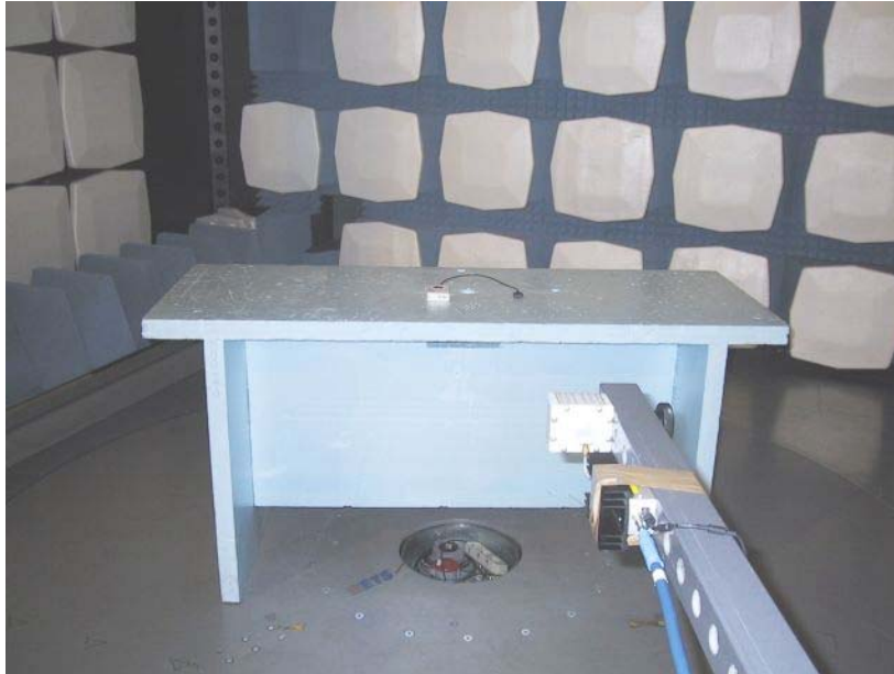
Picture 2: Radiated spurious emission measurement set-up for above 18 GHz measurements, EUT in vertical orientation
