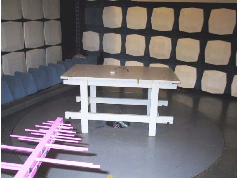
Picture 1: Radiated spurious emission measurement set-up for below 3 GHz measurements, EUT in vertical orientation
