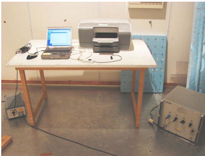
Picture 4: Conducted emission measurement setup
