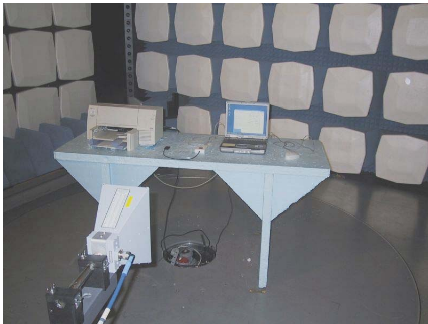
Picture 3: Receiver radiated emission measurement set-up.
