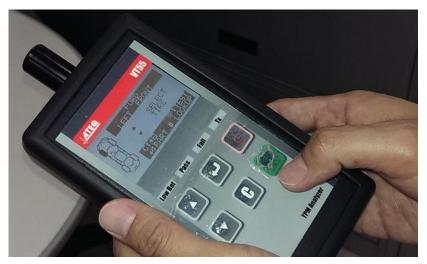
(5) Trigger the sensor (press the TEST button)
