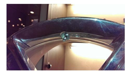
Hold the sensor body against the rim and install then tighten the screw to 20 in-lb
