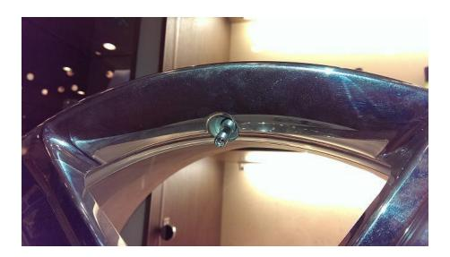
Hold the sensor body against the rim and install then tighten the screw to 20 in-lb Mount the tire back to vehicle
