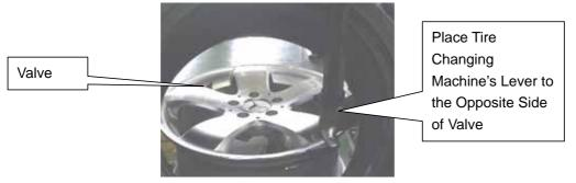
2nd. Use auto-install machine to install the lower-side of tire onto rim.
