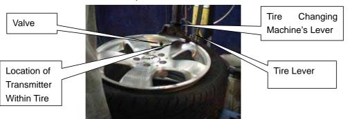
**2nd.** Place the machine Tire Lever on the tire bead and lift tire bead with a manual Tire Lever over the installation head and pull tire away.
