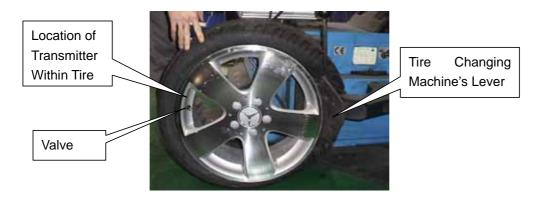
**Caution:** In order not to damage the transmitter , Tire Level should be placed in the opposite side of valve<sub>o</sub>
