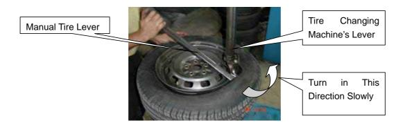
**3rd.** Utilize Manual Tire Lever , simultaneously with Tire Changing Machine's Lever , to pull the lower tire bead away from upper side of wheel.
