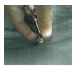
2. Hold the sensor body against the rim and install then tighten the screw to 20 in-lb (2.2 N.m)
