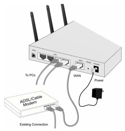
Figure 3: Installation Diagram
