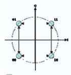
Signal doesn't cross zero, because only one bit of the symbol is changed at a time
