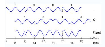
Timing diagram for OQPSK.
