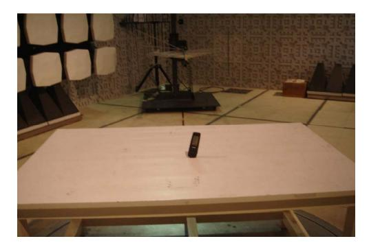
**Radiation Emission Test View For 1GHz-5GHz**
