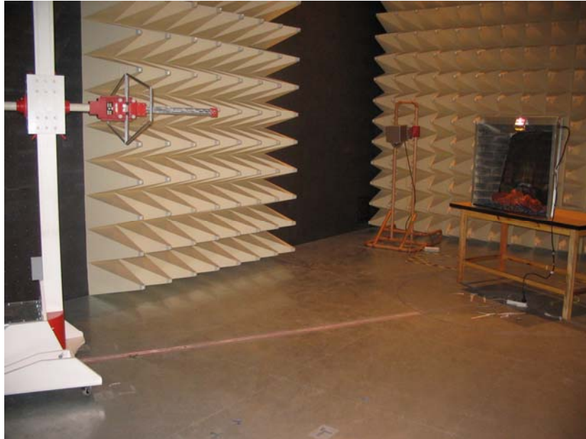
Photograph 2: Set-up for spurious radiated emissions
