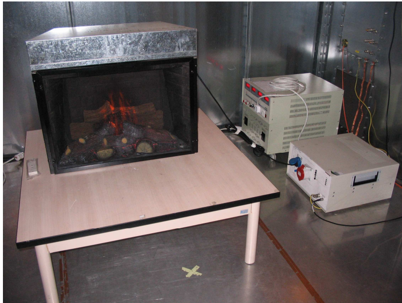
Photograph 1: Set-up for conducted emissions
