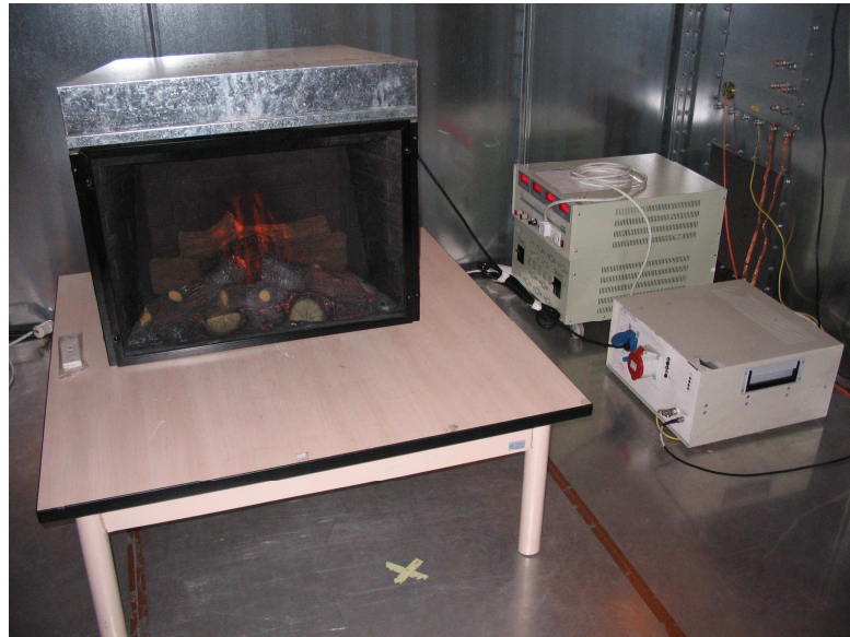
Photograph 1: Set-up for conducted emissions
