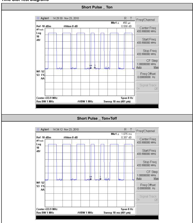
The EUT was complied with the requirement of FCC 15.231 (a) (1), which employed a switch that will automatically deactivate the transmitter within less than 5 seconds of being released.
