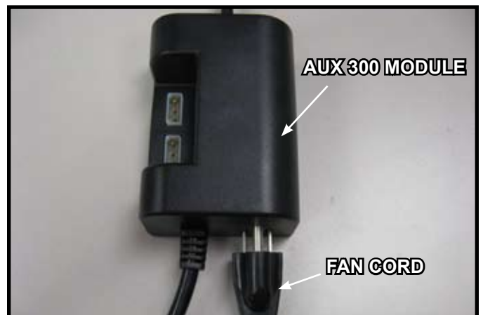
Figure 6. Plug Fan into AUX300 Module
