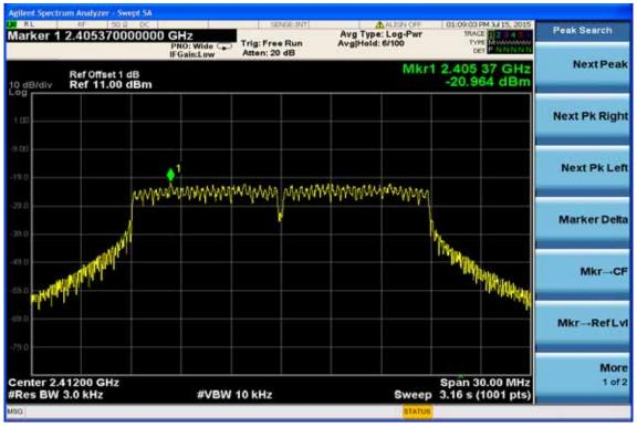
**Power Spectral Density Test Plot (CH-Mid)**
