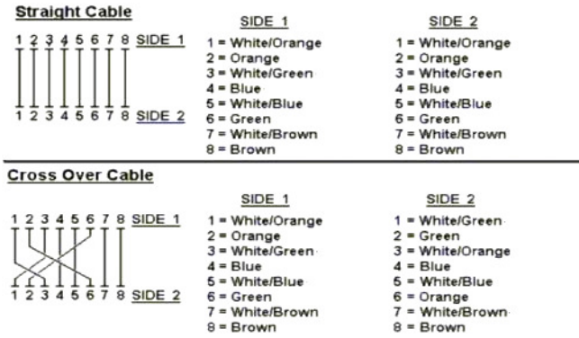
Figure A-1: Straight-Through and Crossover Cable
