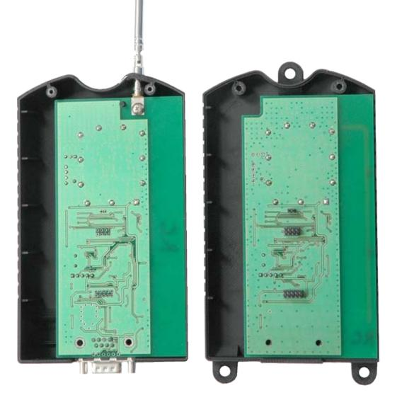
Model: Robot Controller Internal Photo Master Board, Component Side
