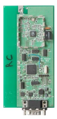
Model: Robot Controller Internal Photo Slave Board, Component Side Shield Cover Removed
