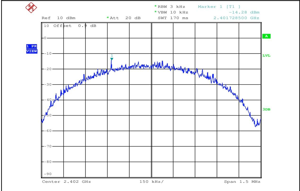
Maximum Peak power spectral density\_BLE\_2440\_Ant1
