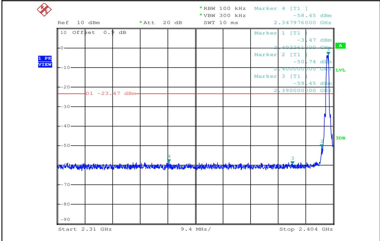
**Band-edge for RF Conducted Emissions\_BLE\_2480\_Ant1**
