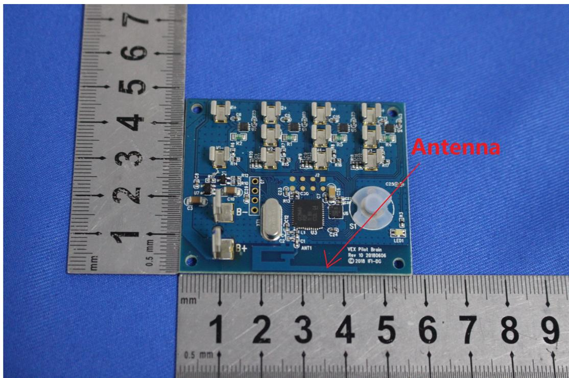
The antenna is integrated on the main PCB and no consideration of replacement. The best case gain of the antenna is 3.3dBi.
