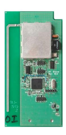
Model: Operator Interface Internal Photo Master Board, Far Side
