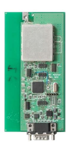
Model: Operator Interface Internal Photo Slave Board, Component Side
