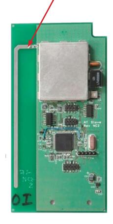
Model: Operator Interface Internal Photo Master Board, Component Side Shield Cover Removed
