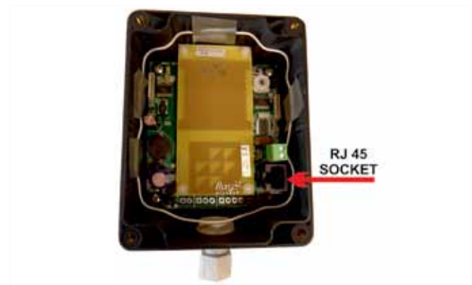
Fig. 33 - RJ45 connection on the Sensor
