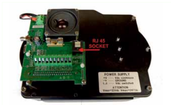
Fig. 32 - RJ45 connection on the CPU
