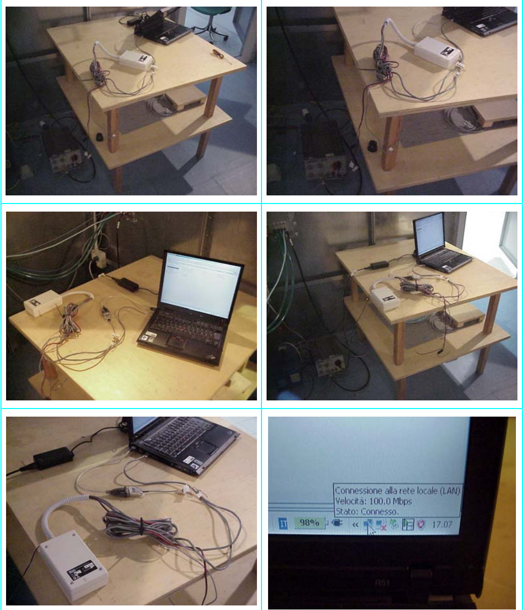
Set-up of Emission Conducted test
