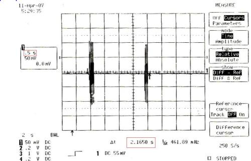
In figure you can see a plot of a transmission of APB mode, with pseudorandom time forced to max and so this is the worst case.
