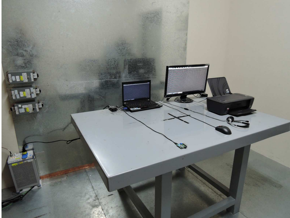
Photograph 6: Set-up for for Mains Conducted testing Front
