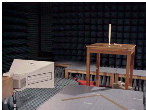
Set up of Radiated emission test
