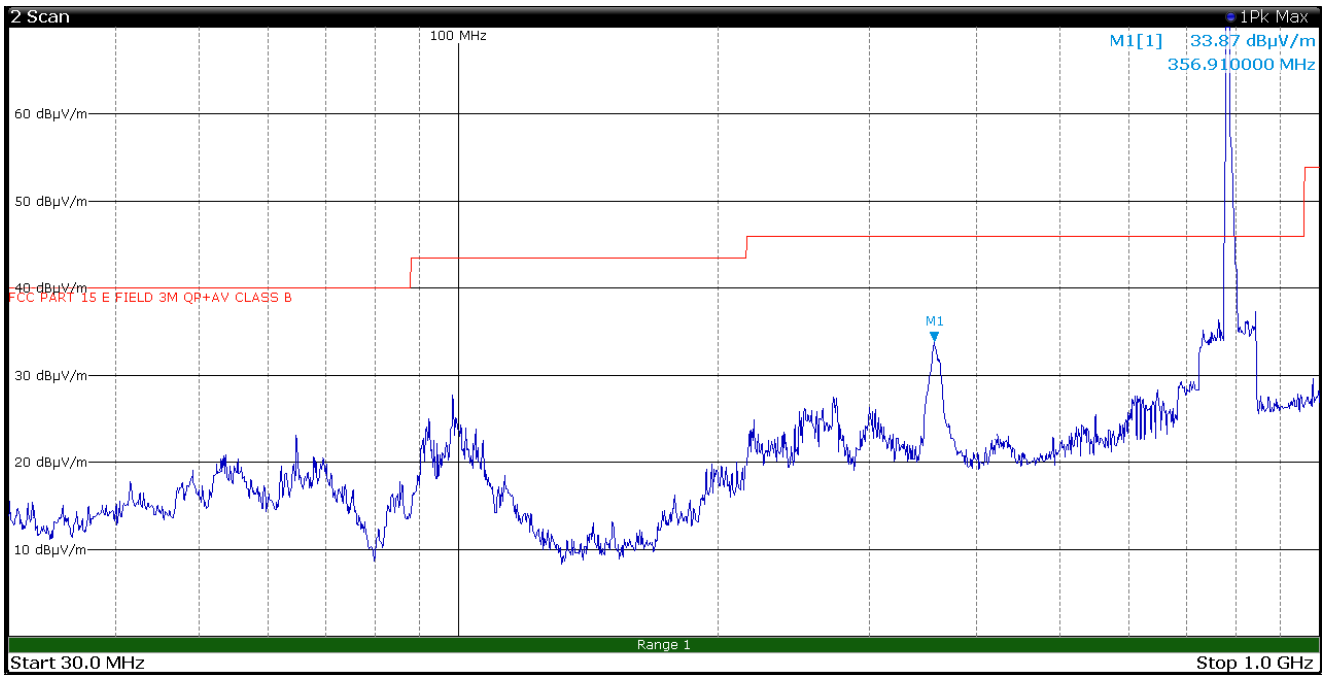
Figure 8.1-105: Radiated spurious emissions, LTE Tx at 782 MHz, WIFI Tx at 5200 MHz – antenna in horizontal polarization – EUT in configuration 2
