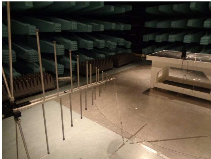
Radiated emission below 1 GHz – Antenna configuration 2
