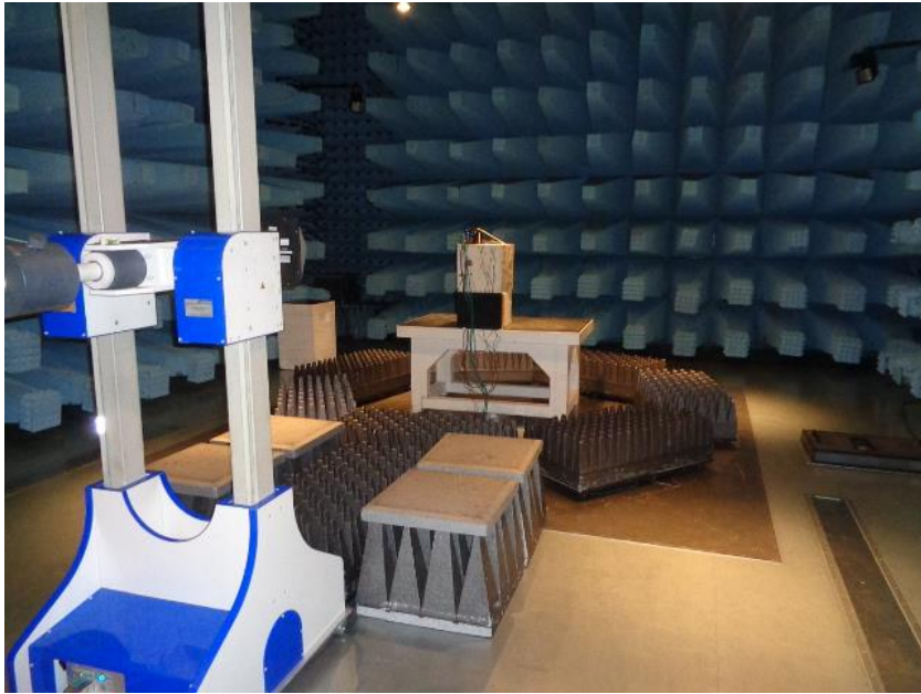
Radiated emission above 1 GHz
