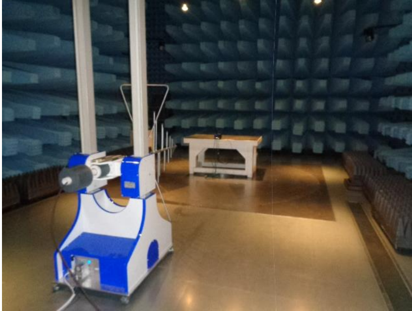
Radiated emission below 1 GHz
