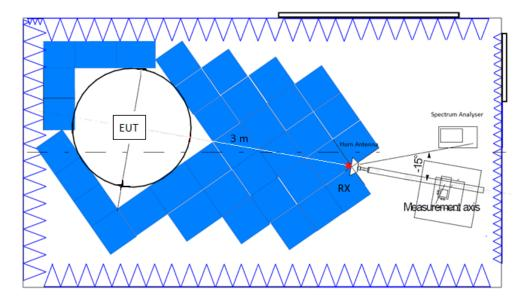
Radiated measurements setup f > 17 GHz:
