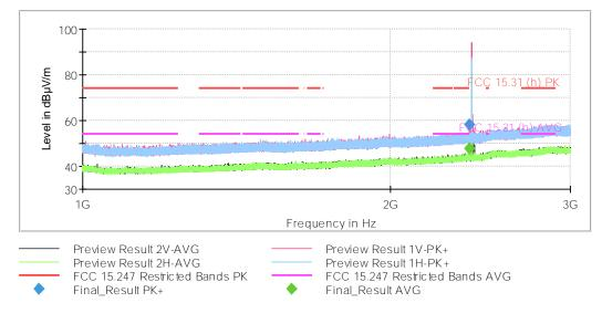
The peak above the limit is the Bluetooth LE carrier frequency.
