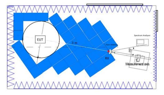
Radiated measurements setup f > 17 GHz:
