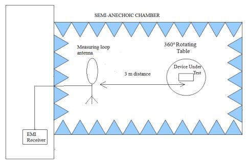
Shielded Control Room For Radiated Measurements
