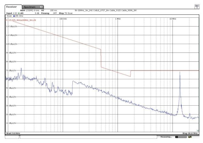
The highest peak is the RFID 13.56 MHz carrier frequency.
