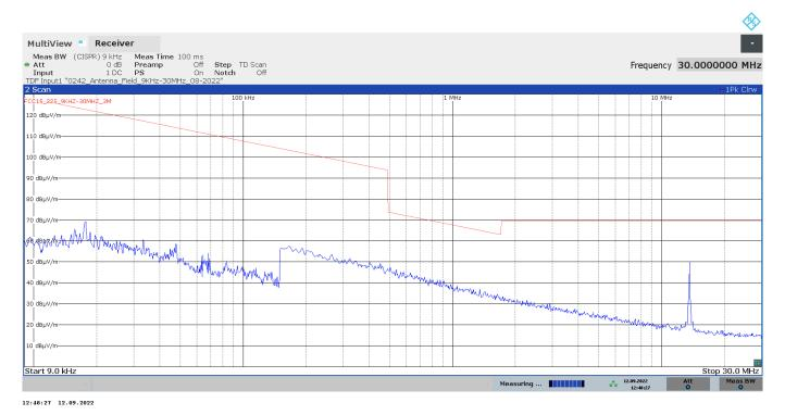
The highest peak is the NFC 13.56 MHz carrier frequency.
