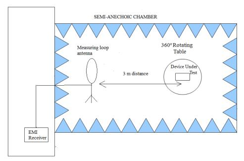
Shielded Control Room For Radiated Measurements
