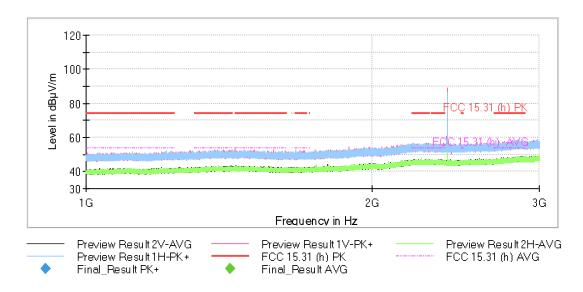
The peak above the limit is the Bluetooth LE carrier frequency.
