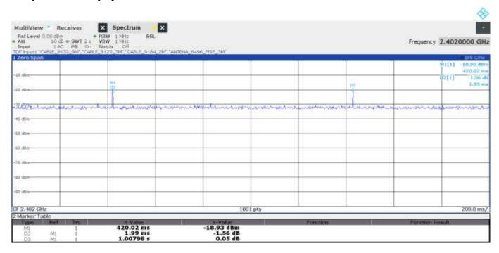
According to ANSI C63.10, paragraph 7.5, we can determinate the Duty Cycle in this way: Duty cycle correction factor  $\delta$  = 20 \* log (Tx ON (ms) \* Number of pulses within 100 ms) / 100 ms  $\delta$  = 20 log (1.99ms/100ms) = -34.02 dB.
