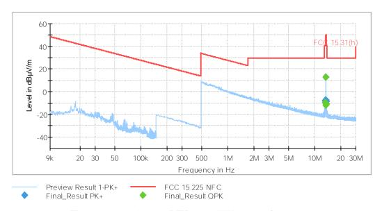
The highest peak is the RFID 13.56 MHz carrier frequency.
