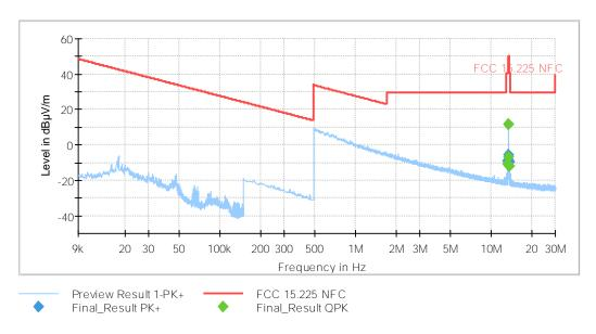
The limits shown in the above plot are extrapolated to 3 meters. The highest peak corresponds to the carrier level.
