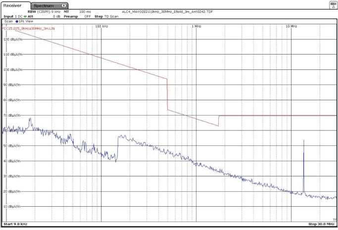
The highest peak is the RFID 13.56 MHz carrier frequency.
