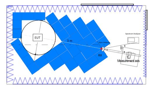
Radiated measurements setup f > 17 GHz:
