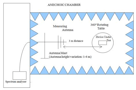
$Shielded\,Control\,Room\,For$ Radiated Measurements
