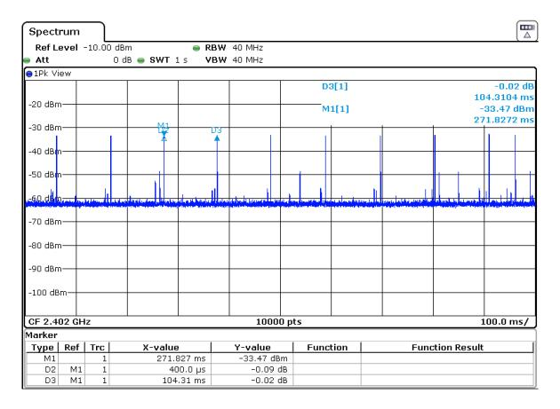
According to ANSI C63.10, paragraph 7.5, we can determinate the Duty Cycle in this way: Duty cycle correction factor  $\delta$  = 20 \* log (Tx ON (ms) \* Number of pulses within 100 ms) / 100 ms  $\delta$  = 20 log (400us)/100ms = -47.97 dB.
