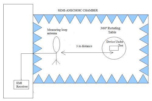
Shielded Control Room For Radiated Measurements
