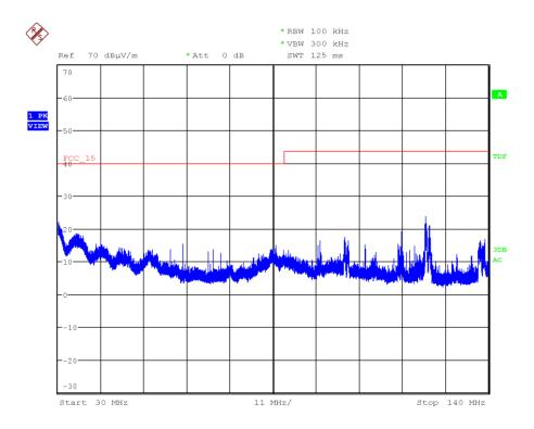
Note: The above plot shows the results of the scan using peak detector.
