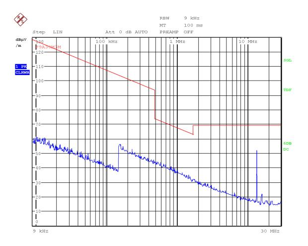
Note: The limits shown in the above plot are extrapolated to 3 meters. The highest peak corresponds to the carrier level.
