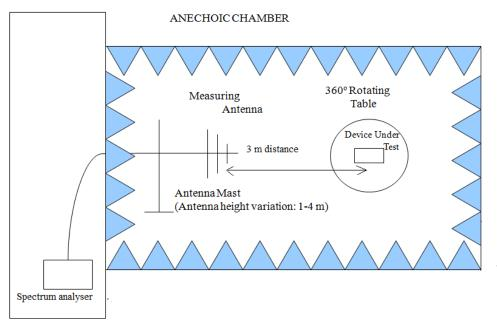
Shielded Control Room For Radiated Measurements
