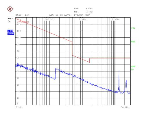
Note: The limits shown in the above plot are extrapolated to 3 meters. The highest peak corresponds to the carrier level.
