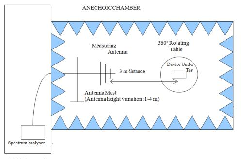
Shielded Control Room For Radiated Measurements
